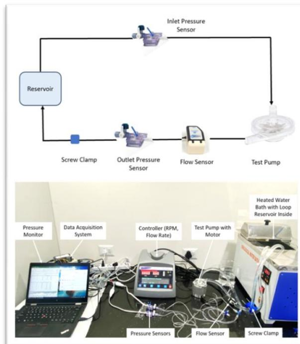
Figure 2 Mock circulatory loop for Hydrodynamic Test.
