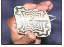
size) is via the use of fractal geometry, which gives rise to **fractal antennas**.
